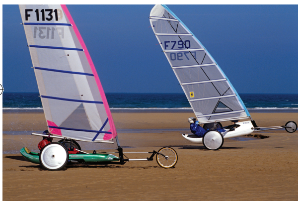
Figure 8.29 The wind passing in front of the sail is fast enough to experience a significant reduction in pressure and the sail is pulled forward
